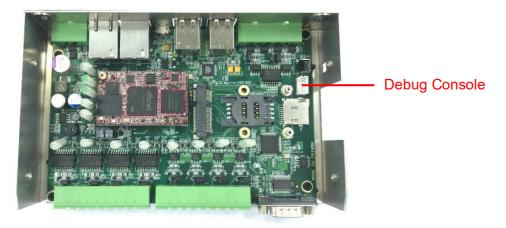
Pin assignment is: RX, TX, +3.3V, GND.
