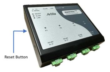
The behavior of the reset button depends on how long you press the reset button.
