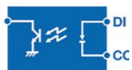
2500Vrms Opto-isolation Digital Input
