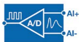
16-bit A/D Converter Diff. input, mV, V, 0~20mA
