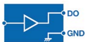
500mA High-Drive Digital Output
