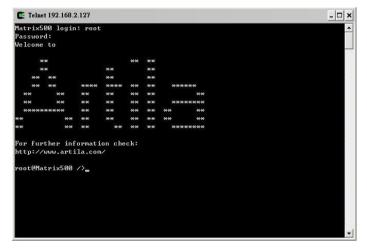
To compile the example program, simple use the Makefile of the example program and type *make clean* to clean the execution file that had been built and then type *make* to compile the new execution file
